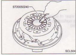
Adjust unevenness of diaphragm spring with Tool.
