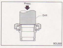
Install release bearing with suitable drift.
