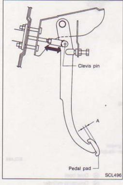
Adjust pedal free play with master cylinder push rod. Then tighten lock nut.
